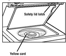
**STEP 2.** Pull the styrofoam packing out of the washer.
